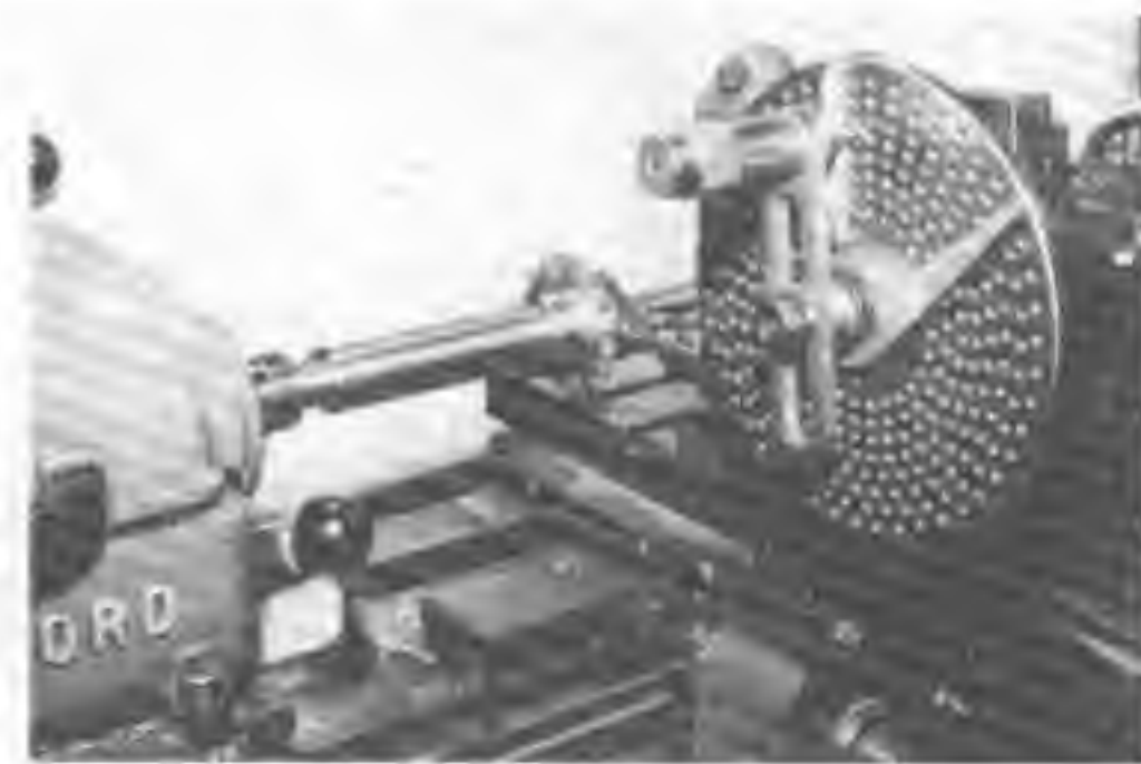
Fig. 61 Centralising the cutter. The vertical slide has been set at a low angle to allow the centre access to the cutter.
